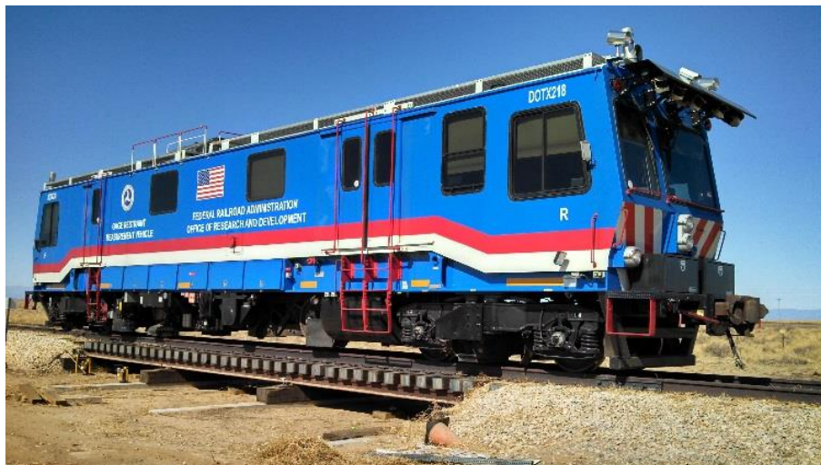
Rys. 12: Pojazd do pomiaru toru na BDTF (Bridge Deflection Test Facility)
